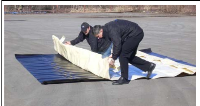
Folding the berm liner.
