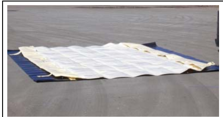
Berm liner laid flat.
