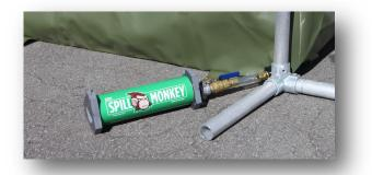
**Step 1** – Attach the  $\frac{3}{4}$ " NPT sight glass connection to the berm. The sight glass has been designed to eliminate the chance of releasing contaminated water into the local environment. Quality material has been used to ensure uninterrupted filtration.
